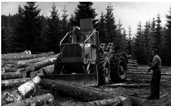
The Kockum tractor was the precursor of the more widespread usage of heavy equipment in the forests (photo Krkonoše National Park Administration archive)
